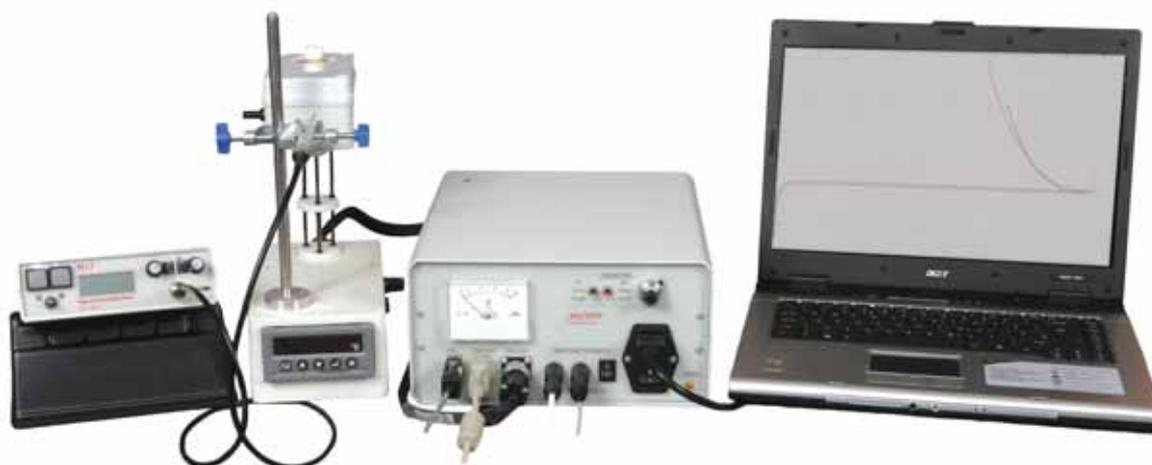
This system is used in the investigation of magnetic mineralogy and grain size and for the determination of Curie transition temperatures. It permits magnetic susceptibility measurements to be made on 15mm diameter (2.5ml) samples over the temperature range -200°C to +850°C.
