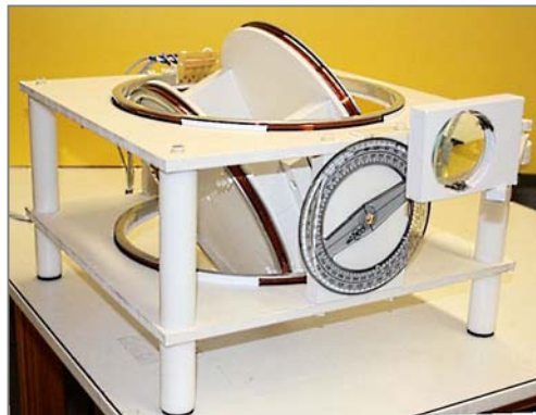
Fig. 2: Apparatus to measure M in function of angle, on pairs of about 300-mm in diameter.
