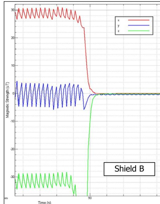
**Commentaries:** For such simple shields, with open ends, made in minutes, with a cost of less than 70 Euro each, we can say that the results are good and useful in many practical cases. The attenuation would be greater in higher strength fields, up to 100 or 200  $\mu$ T, since the material would operate with higher magnetic flux and permeability, without reaching saturation.
