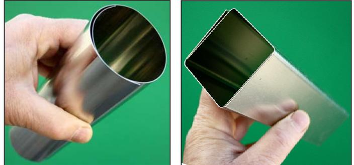
**Screen B:** Of rectangular cross section, with interior sides of 53 x 50 mm, and length of 210 mm. This is made from two "U" shaped pieces each one made with a half of a CP020-A4 sheet. The pieces were bent by hand on a square tube of 50 x 50 mm, with rounded edges. The interior bend radius is about 2 mm.
